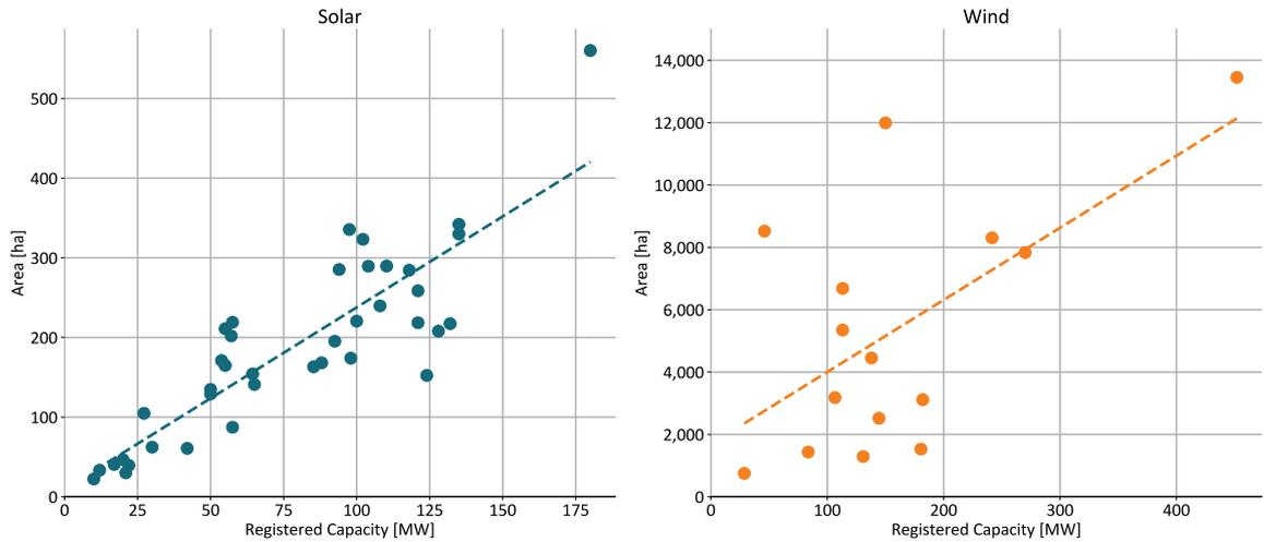
Figure 10. Correlation between registered capacity and area of solar and wind generators with line of best fit
