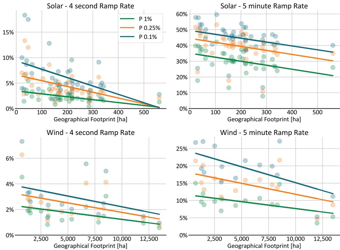
Figure 9. The relationship between normalised ramp rate exceedance probabilities and geographical footprints (convex hull)
