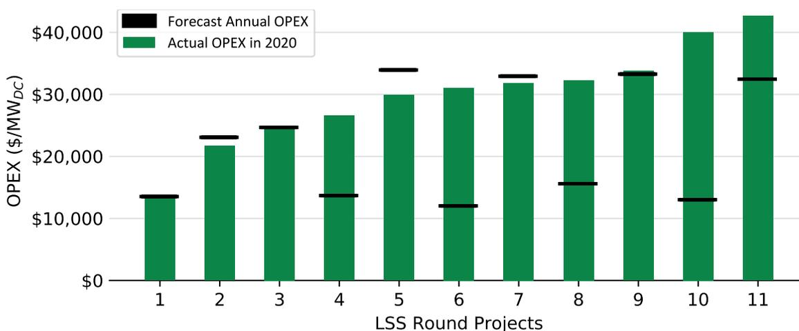
Figure 11. Bar chart showing actual OPEX in 2020 for 11 of the LSS Round Projects. The respective forecast OPEX for each project is displayed by a horizontal black line.
