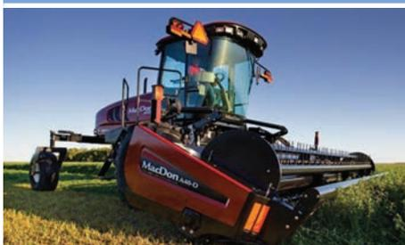
A new windrower helped a family business in Ballarat, Victoria reduce diesel consumption by about 25 per cent, cut carbon emissions and improve energy productivity. The windrower saves 2 to 2.5 litres of diesel per hectare.
