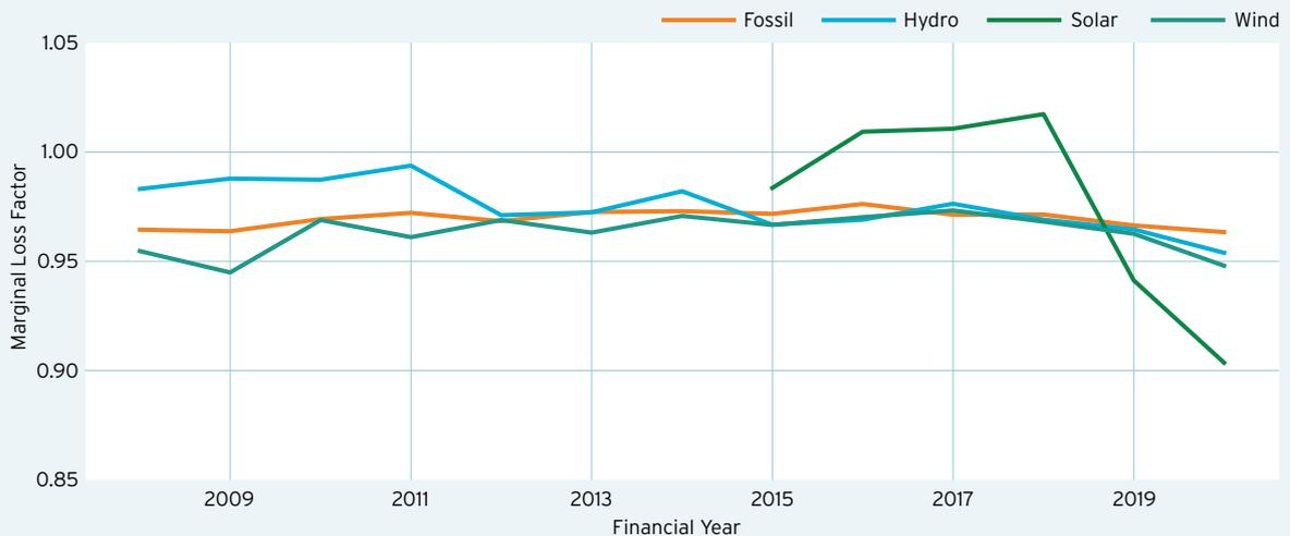
**Figure 14. The weighted average (weighted by nameplate capacity) MLF for generator technologies on the NEM (according to current records from AEMO for all generators greater than 5 MW)**
