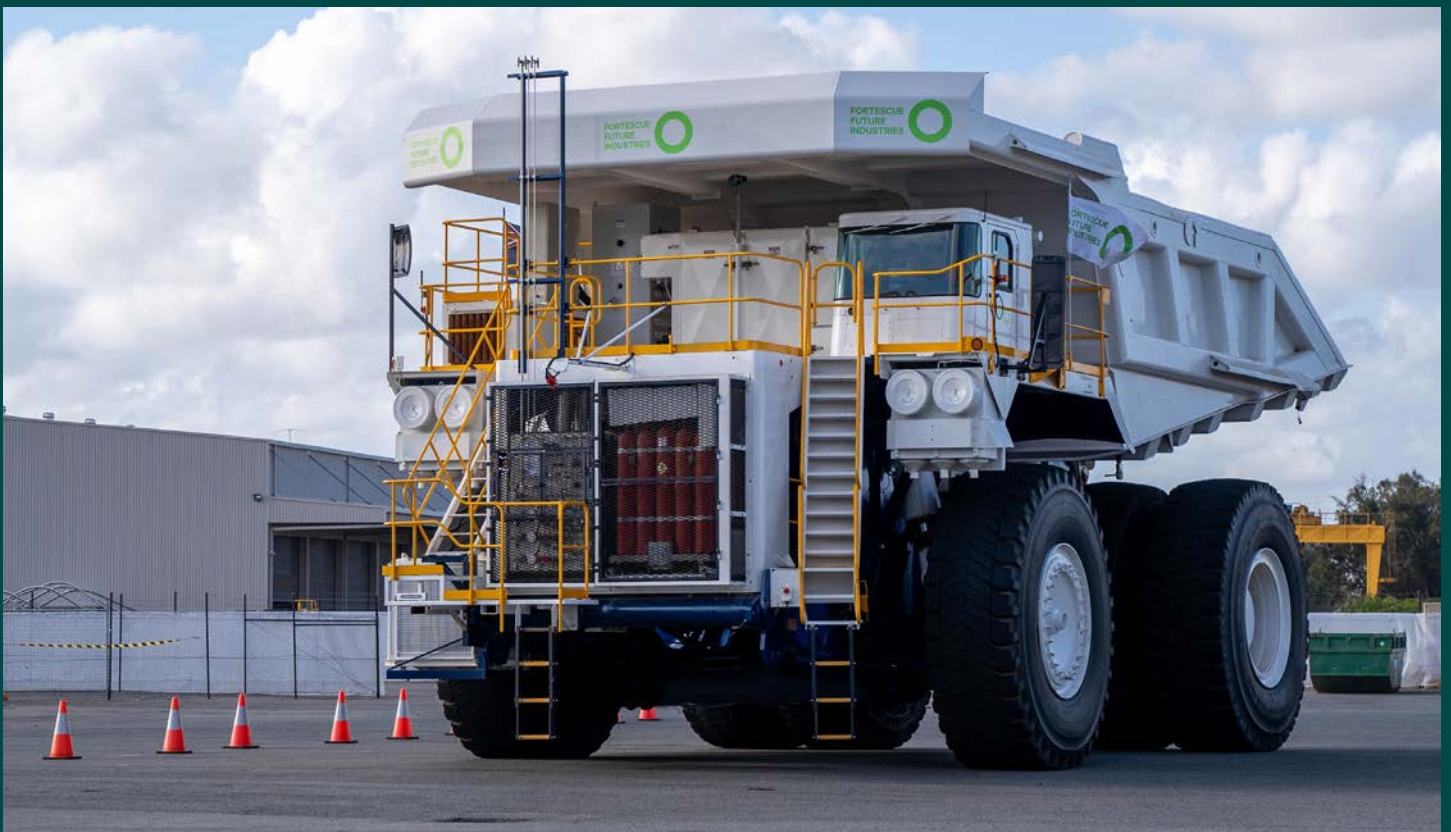
Figure 14 FMG hydrogen haul truck trial (image courtesy of FFI).
