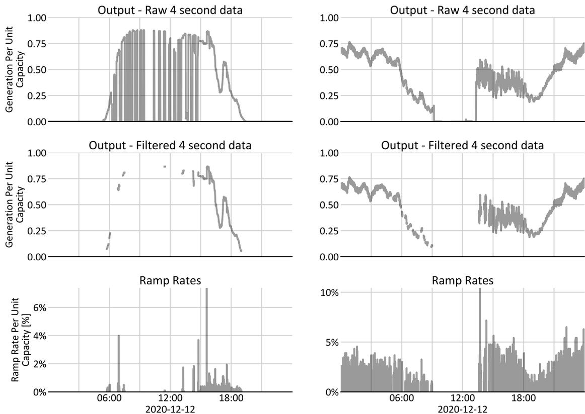
Figure 1. Process of filtering normalised ramp rate data and calculating 4-second ramp rates for solar (left) and wind (right) farms
