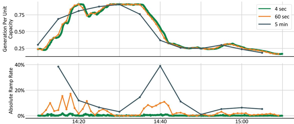
Figure 2. Ramp rates at four second, one minute and five minute frequencies over a one hour period for a solar farm
