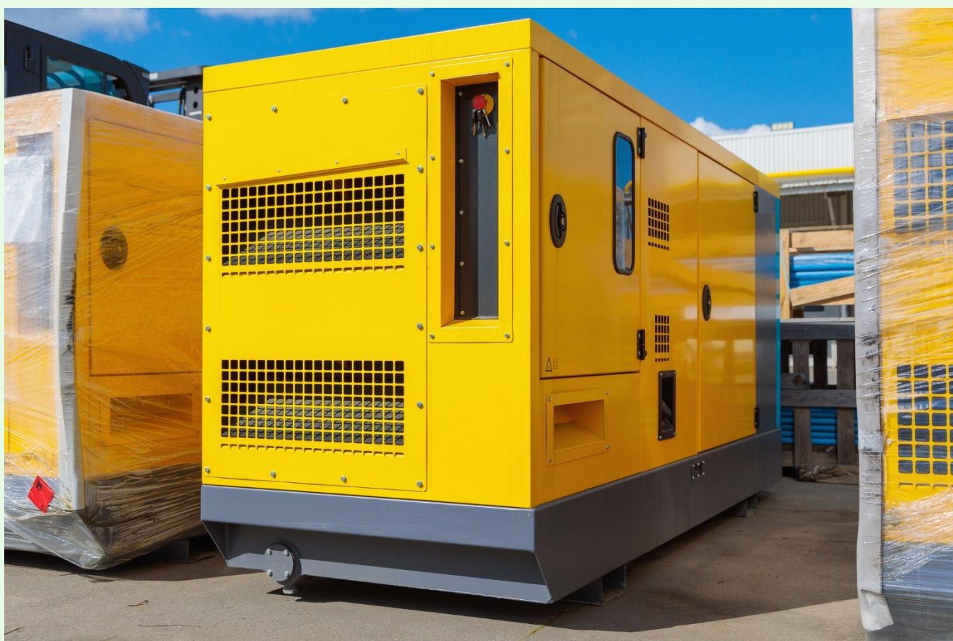
Figure 13: Diesel generators using reciprocal engines to convert chemical energy into electricity
