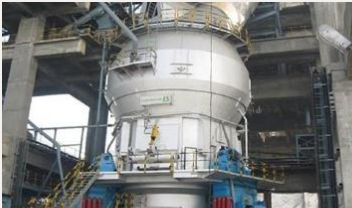
Figure 56: Vertical roller mill at West Musgrave mine (image courtesy of OZ Minerals)
